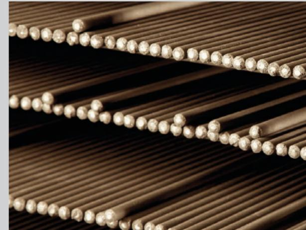
VAUTID hardfacing material as stick electrodes
