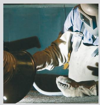
Manual hardfacing using VAUTID stick electrodes
